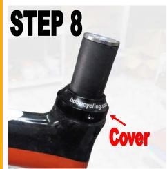
**STEP 8:** Slide on the cover and any spacers you want. Be sure to orient the hole on the cover with the bolt on the collar.
