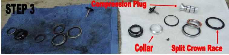
**STEP 3**: Lay out the old headset parts and inspect. Look for any odd or uneven wear patterns as indications of possible misalignment or damage. Do a quick inspection of the fork and steerer tube as well. Prepare the new headset for installation.
